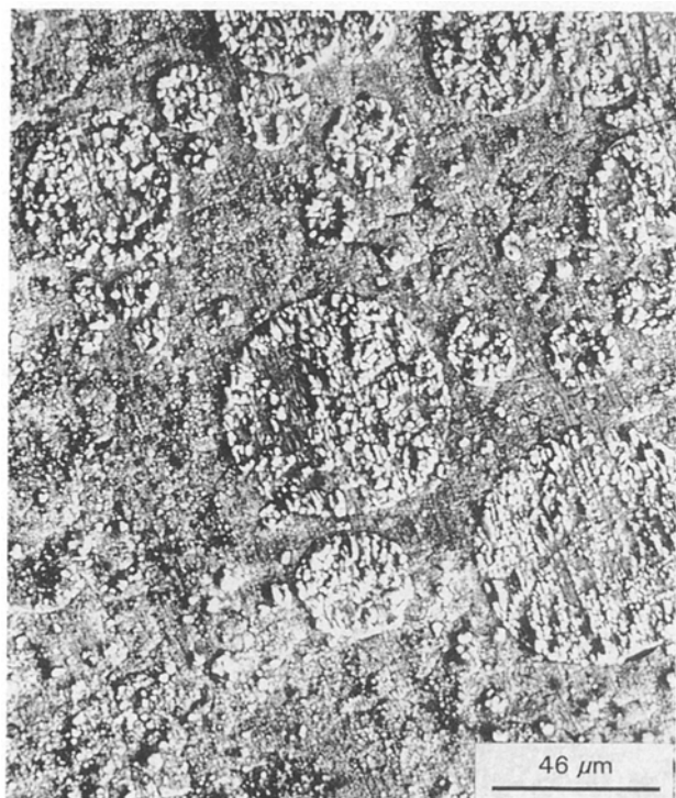
Figure 6 View of the nanonickel surface with conglomerates of powder particles precipitated from the evaporated droplets of mercury.
