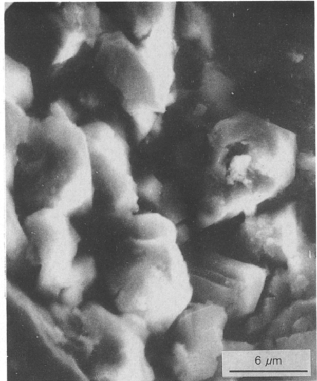
Figure 3 Minute view of zone II (zone of subcritical fracture growth).
